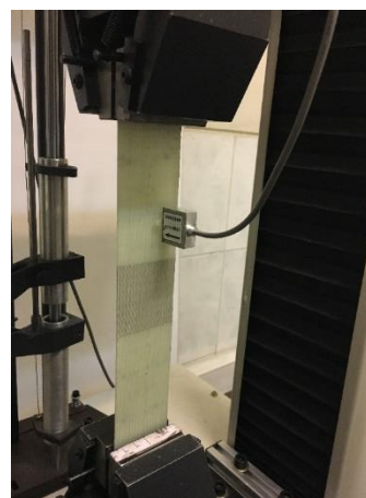
Fig. 7 Attaching the accelerometer to the specimen
