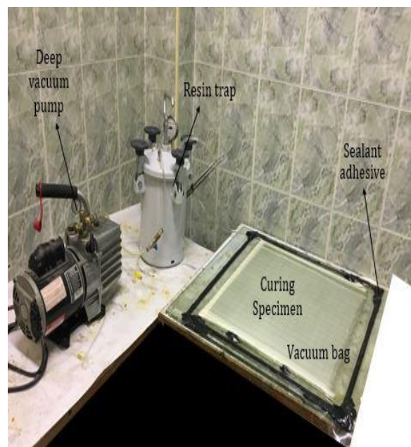
Fig. 3 Specimen manufacturing process
