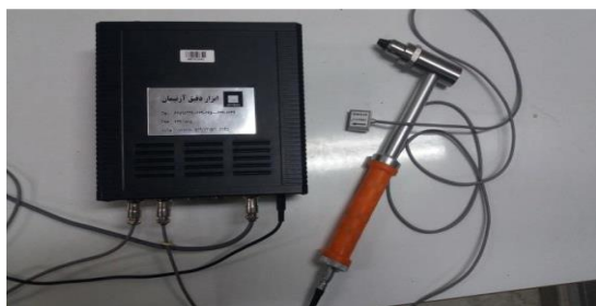
Fig. 8 Analyzer, accelerometer and excitation hammer
