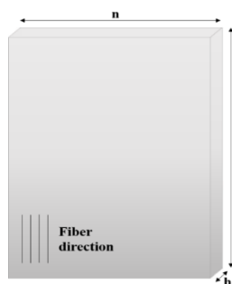
Fig. 2 Schematics of a flat plate sample.
