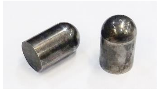
Fig. 2 Hemispherical projectile used in experiments
