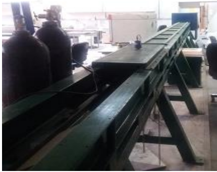
Fig. 3 Gas gun used for ballistic tests
