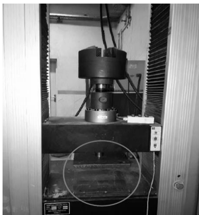
Fig. 5 Image universal testing machine for conducting a pressure test between two parallel rigid plates
