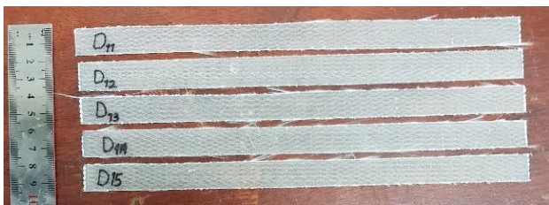
Fig. 1 Composite samples of stress relaxation test
