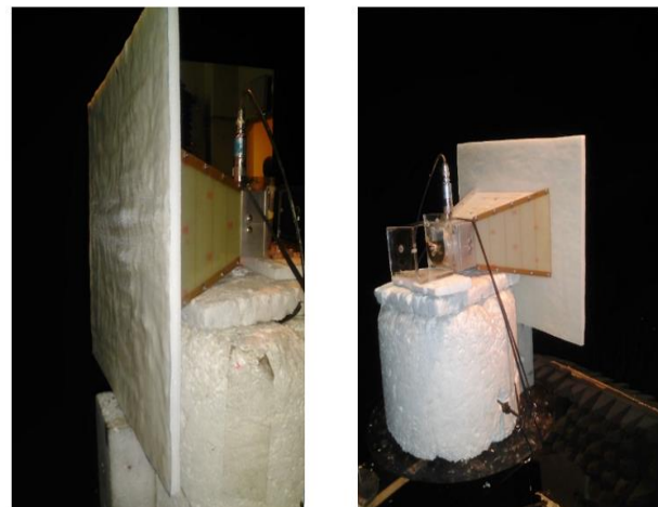
Fig. 18 Test set – up for free space test in the antenna lab.
