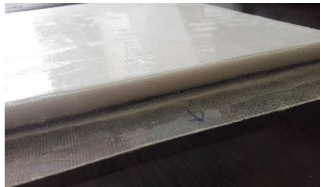
Fig. 17 Hand lay – up made sandwich panel sample prepared to electromagnetic tests
