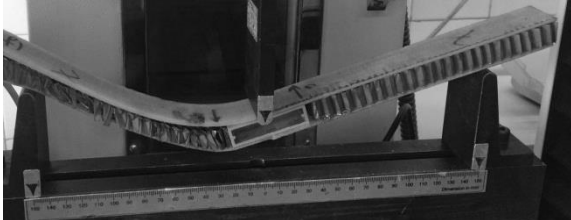
Fig. 13 Shear deformation and buckling of honeycomb after performing bending test on the beams with connection type 2
