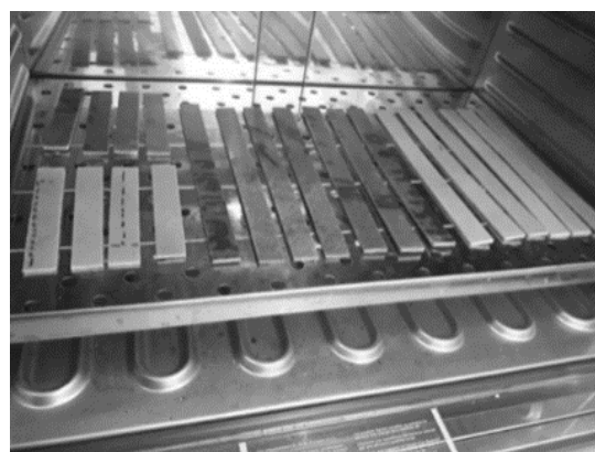
Fig. 3 Post-cure process of the specimens
