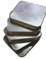
Fig. 8 Sintered Specimens at 530°C
