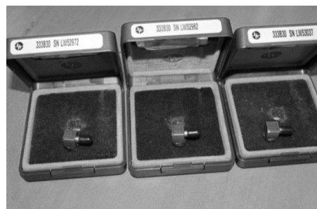
Fig. 3 sensor that used in modal test
