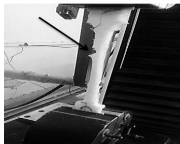
Fig. 9 Start of failure from sample surface during tensile test
