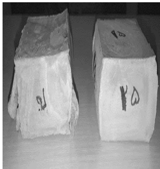
Fig. 5 Polyurethane foam samples under uniaxial compression test
