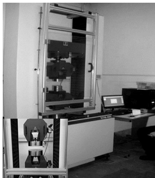
Fig. 8 A view of the Santam tension and compression testing machine
