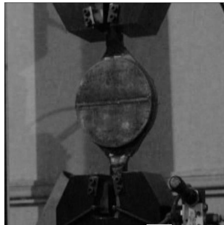
Fig. 16 Mechanical tensile test of the Nol ring
