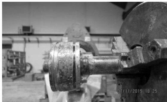
Fig. 9 Filament winding process of the nol rings
