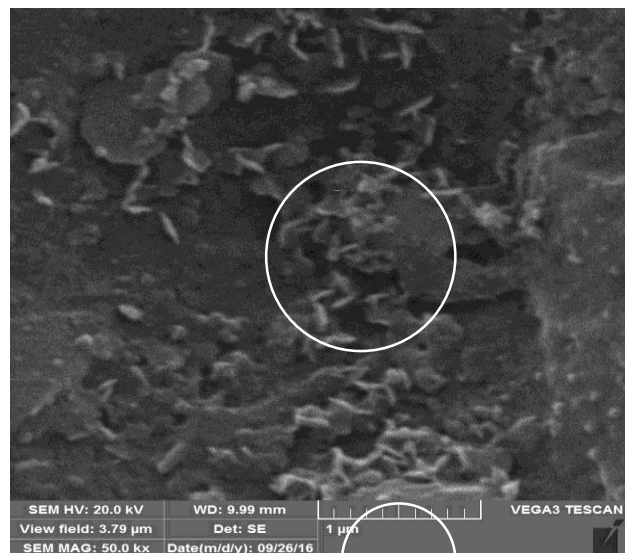
Fig. 15 Scanning electron microscope image of the carbon nanotubes agglomeration mechanism in nanocomposite reinforced with 1 Wt%
