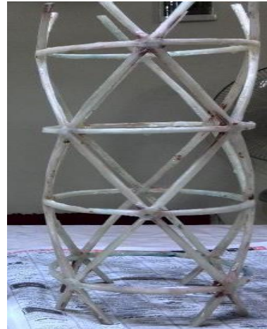
Fig.4 Lattice sample made using Teflon mold
