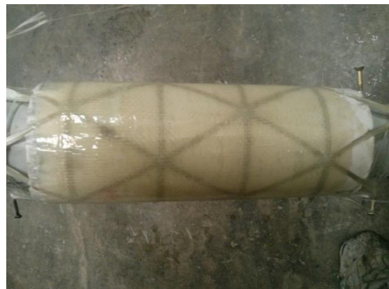
Fig. 9 Lay up of skin around ribs
