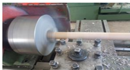
Fig. 2 machining of surface of mandrel for sizing
