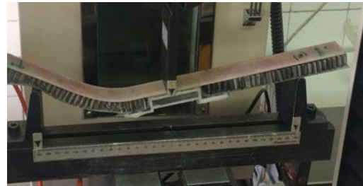
Fig. 11 Shear deformation and buckling of honeycomb after performing bending test on the beams with connection type 1
