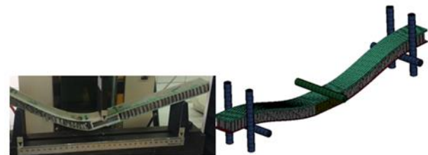
Fig. 24 Failure modes after performing bending test on the beams with connection type 2 (Numerical and experimental)
