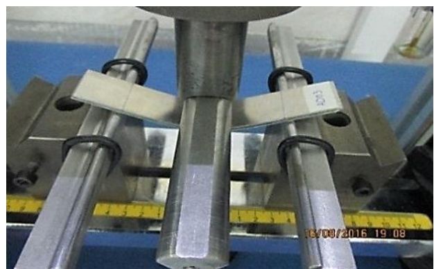
Fig. 3 Three-point bending test.
