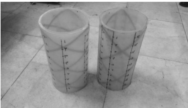
Fig. 6 Composite sandwich shell with lozenge core
