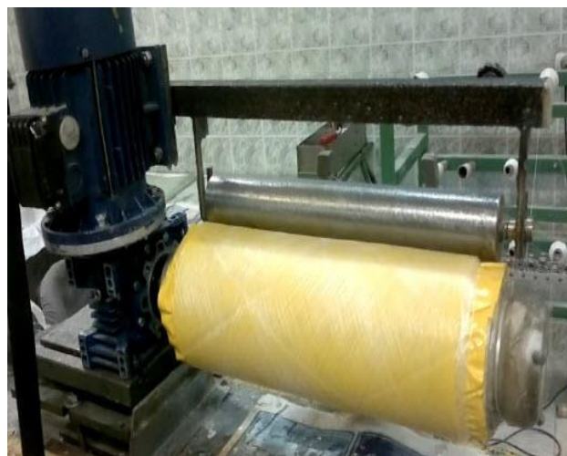
Fig. 3 Filament winding process
