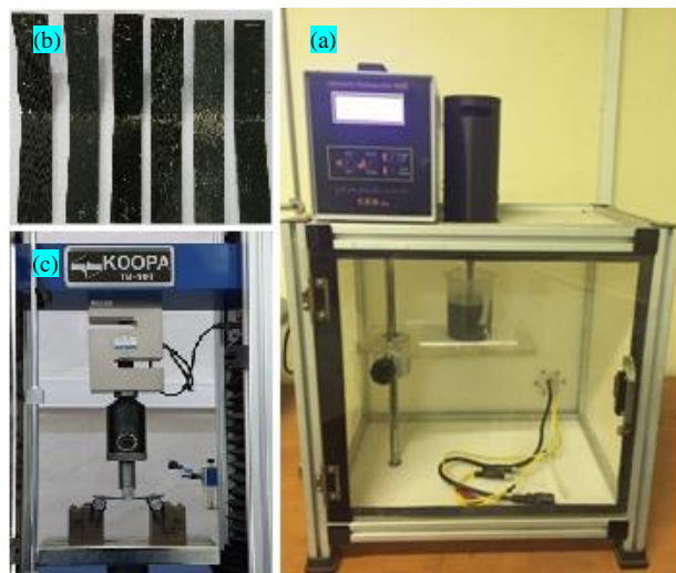
Fig. 2 Dispersing of graphene in epoxy and testing of bending samples. a) Ultrasonic operation, b) A number of tested bending samples and c) three-point bending test.
