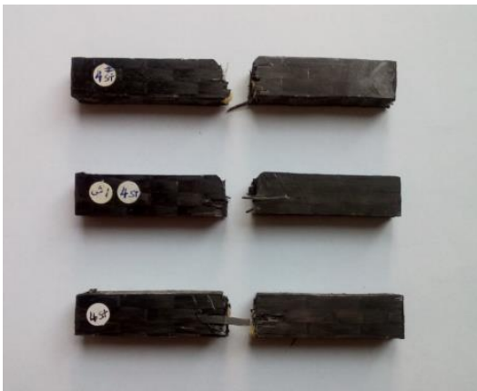
Fig. 6 Sandwich panel specimens with 4 pairs of self-healing micro tube after CHARPY impact test
