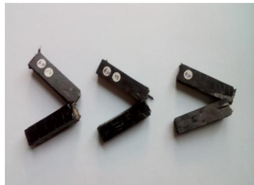
Fig. 7 Sandwich panel specimens with 6 pairs of self-healing micro tube after CHARPY impact test
