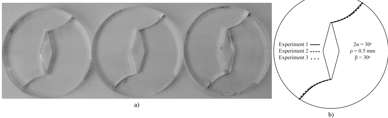
Fig. 3 Verifying the repeatability of the experiments for constant geometrical and loading conditions
