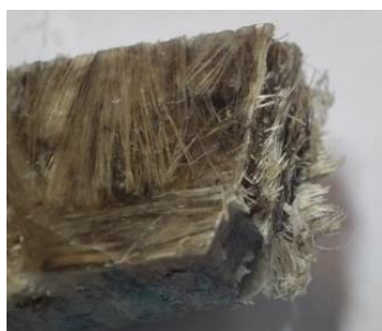
Fig. 9 Impact fractured surface of polyester/kenaf filled with 20 wt% of 1 cm fibers
