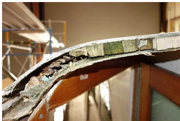
Fig. 1 The life cycle of balsa core: On the right side of the sandwich panel, the core material has retained its original color and strength. The core in the middle has been exposed to moisture and shows early signs of degradation. The core on the left side has decomposed and lost all of its strength [13].
