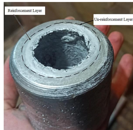
Fig. 1 Al-15Mg 2 Si FGMs tube
