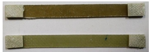
Fig. 1 The fabricated mat and woven composite specimens.
