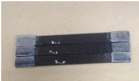
Fig. 9 Multi-layer composite samples for tensile testing
