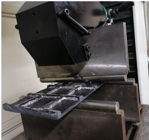
Fig. 8 Perform three-point bending test
