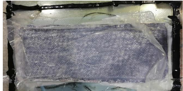
Fig. 5 Using the vacuum method to drain excess air and resin
