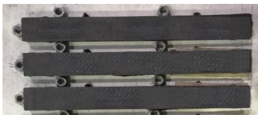
Fig. 13 Samples prepared for DCB and ENF tests
