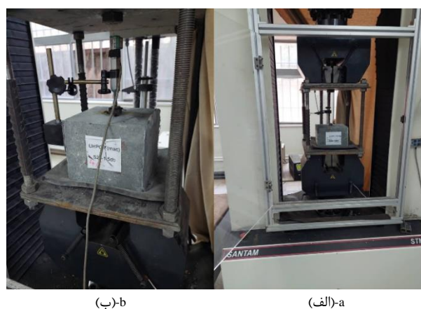
Fig. 4 (a) Test set up details (b) displacement sensor
