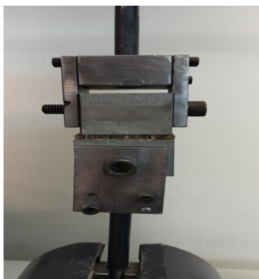
Fig. 1 Sample test of composite plate tension with honeycomb core
