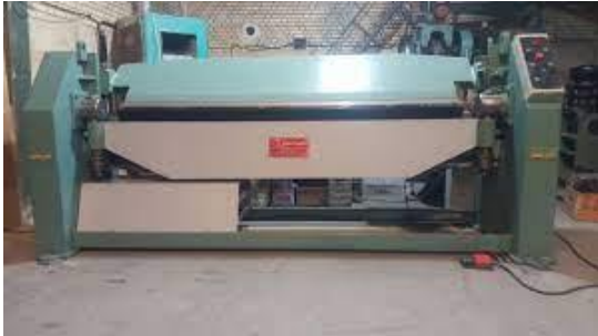
Fig. 1 Bending machine to shape the aluminum core
