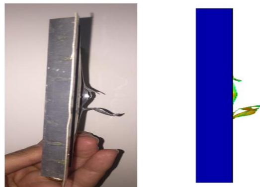
Fig. 26 Core fracture in SGE-3W3 specimen
