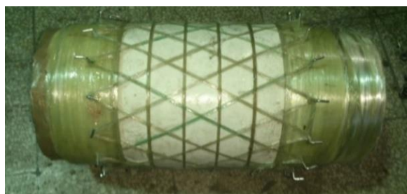
Fig. 5 Composite lattice cylinder (glass-epoxy) wound into a silicone mold on a foam mandrel after curing and before separation from the mold
