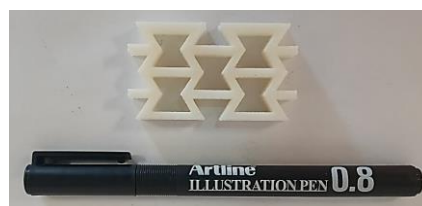
Fig. 2 As printed auxetic structure used for experiment.
