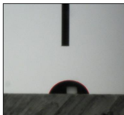
Fig. 15 Photograph of a contact angle test between polymeric sample and water.
