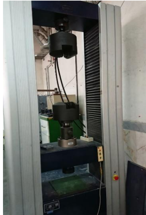
Fig. 4 universal test apparatus for quasi-static test
