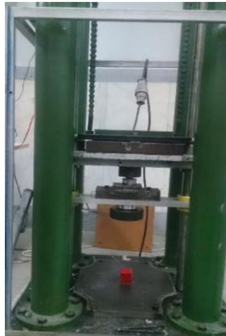
Fig. 5 Drop hammer test apparatus for impact test
