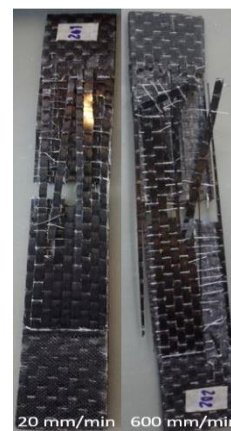
Figure 32 The failure image of tensile samples after testing
