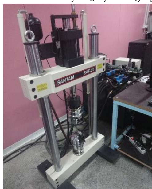
Figure 2 The SAF50 fatigue testing machine, used in this research
