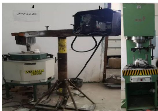
Fig. 1 Experimental setup of (a) casting, (b) extrusion.
