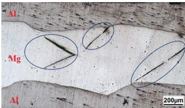
Fig. 10 Optical microscope image of Al / Mg / Al composite layers with shear bands
