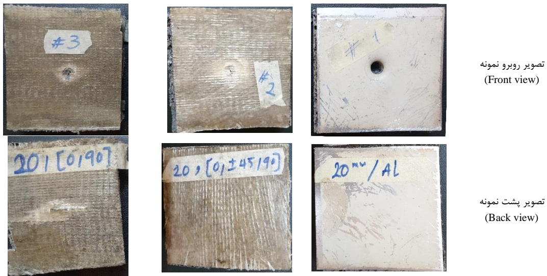
Fig. 13 Front and back view of the specimens after testing by a spherical impactor
