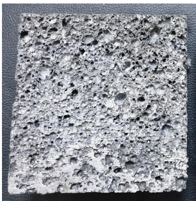
Fig.1 Aluminum foam sample produced
