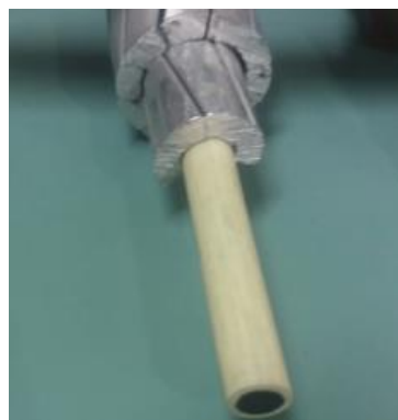
Fig. 1 A high strength low sag conductor consisting of aluminum wires and a hybrid composite core
