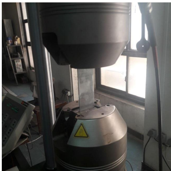
Fig. 2 Fixing test pieces in the fatigue machine
