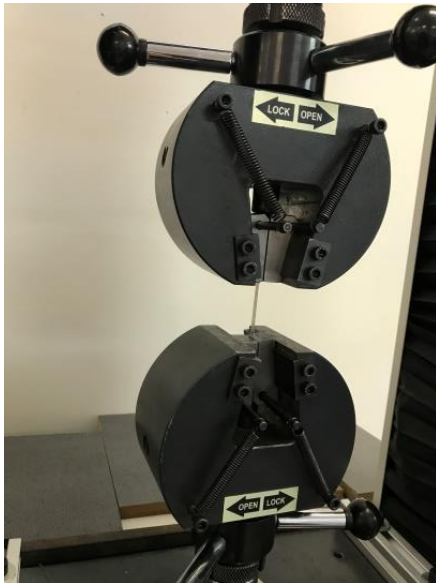
Fig. 3 Image of uniaxial tensile test of aluminum foil
