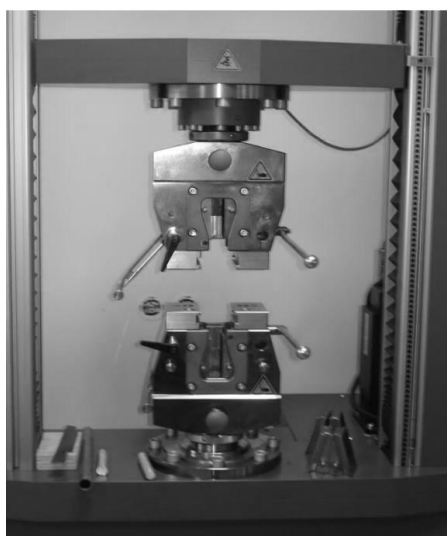
Fig. 3 Tension test for Al and Cu tubes
